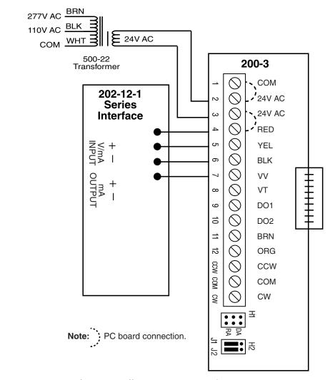
200-3 Flow Controller & 202-12-1 Interface Wiring Diagram
