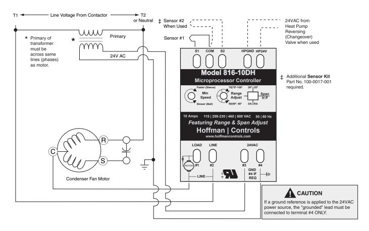
Wiring Diagram for the 816-10DH Figure 3
