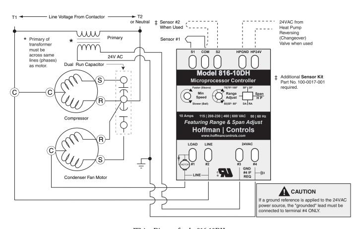
Wiring Diagram for the 816-10DH Figure 4
