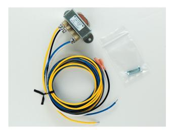
4a. For typical Cooler or Freezer installations, the best way to create a 24Vac power source is to use the Evaporator fan motor 115Vac line voltage power strip and a 115Vac to 24Vac, minimum 4VA transformer or the 24Vac/12VA transformer installation kit as shown below.
