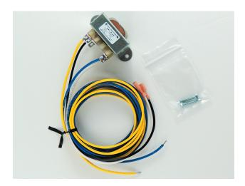
4a. For typical Cooler or Freezer installations, the best way to create a 24Vac power source is to use the Evaporator fan motor 115Vac line voltage power strip and a 115Vac to 24Vac, minimum 4VA transformer or the 24Vac/12VA transformer installation kit as shown below.
