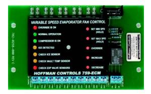
759-ECM Variable Speed Evaporator Fan Control
